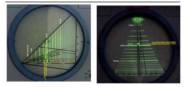
Image 28. Imaging of aircraft position in relation to glide path and RWY center line on WISP-75 displays
