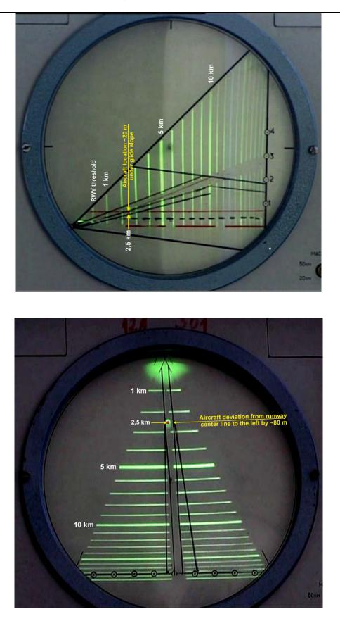
Image 30. Imaging of aircraft position in relation to glide path and RWY 26 center line on WISP-75 displays
