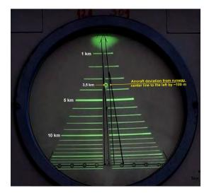
Image 29. Imaging of aircraft position in relation to glide path and RWY 26 center line on WISP-75 displays
