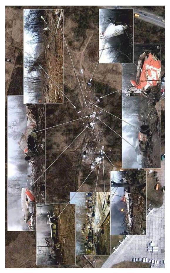
Photo 14. Crash site - location of elements of aircraft wreckage
