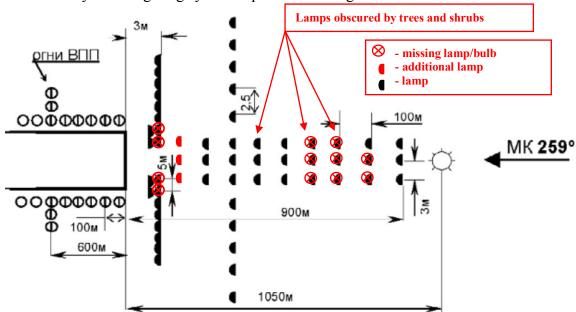
Fig. 15. Serviceabilty of ŁUCZ-2MU lighting system
