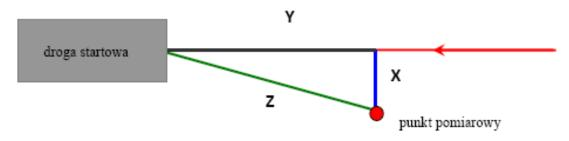
Fig. 12. Graphical scheme which identifies the measurements taken. droga startowa - means runway, punkt pomiarowy – means measurement point
