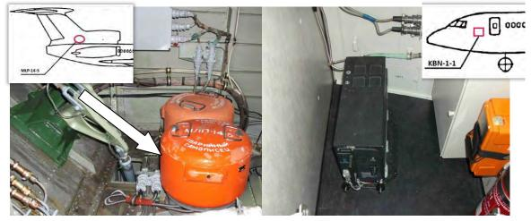
Fig. 10. Locations of crash protected flight data recorder MŁP-14-5 (left photo) and KBN-1-1 (right photo)
