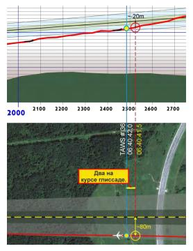
Fig. 29. Location of aircraft at the time command was given: "Два на курсе, глиссаде" ("Two on course, on glide path")
