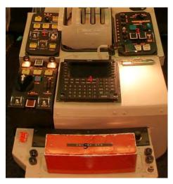
Photo 8. Panels between the pilots' seats (pedestal)
