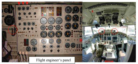
Fig. 12. Arrangement of microphones in the cockpit of Tu-154M
