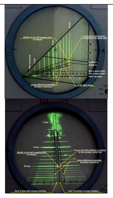
Image 25. Imaging of aircraft position in relation to the glide path an RWY center line on WISP-75 displays
